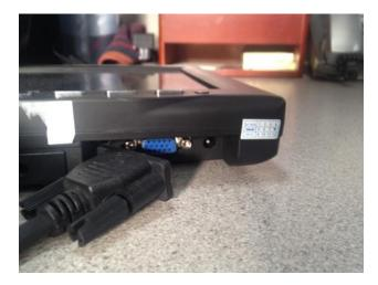
• The above image shows how you would connect the VGA cable, to the VGA port on the bottom of the customer-facing monitor
