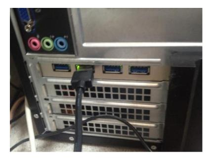
• The above image shows how the USB cable from the SIIG converter will connect to a USB port on your pc
