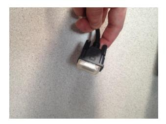
• This is the VGA cable with the plastic cover on. This plastic cover can be removed. Your cable may be blue instead of black.
