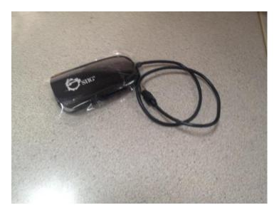
• The above image shows the *SIIG VGA-to-USB converter*. The end of the converter without the USB cable is where you will connect the other end of the VGA cable. The USB cable end will connect to the USB port on your pc.
