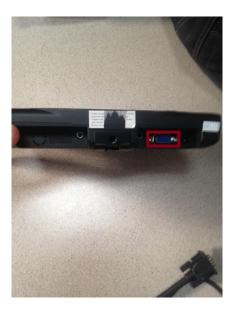
• This is the bottom of the customer-facing monitor – the VGA port is highlighted; this is where you will connect the VGA cable. To the right of the VGA port is the power port, where you would connect the power adapter.
