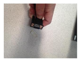
• This is the VGA cable with the plastic covering removed, exposing the connector pins.
