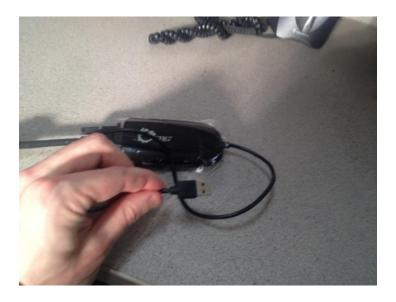
• Next, take the USB cable end of the SIIG converter and connect it to the pc's USB port. The above image shows the USB end of the SIIG adapter.
