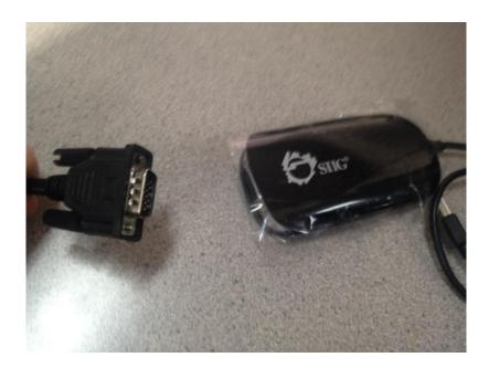
• The above image shows how you would connect the VGA cable to the SIIG converter
