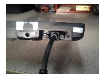
The above image shows the VGA cable completely connected to the bottom of the customer-facing display
